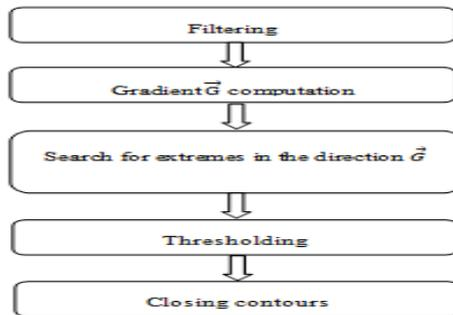
Fig. 5. Flow chart of the Gradient Approach
