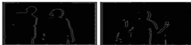
Fig. 11.a Sobel filter applied to the depth images in darkness
