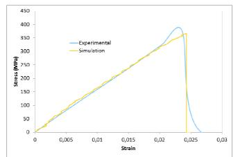
Figure 5. Experimental and simulation curves for quasi-static traction curve at  $0^\circ$
