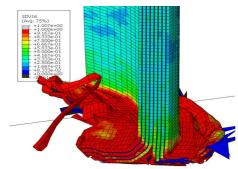
Figure 6. Simulation of drop-weight tower test
