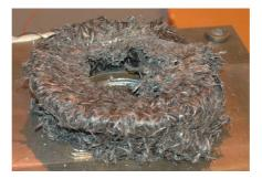
.Figure 3. Picture of the splaying mode of energy dissipation
