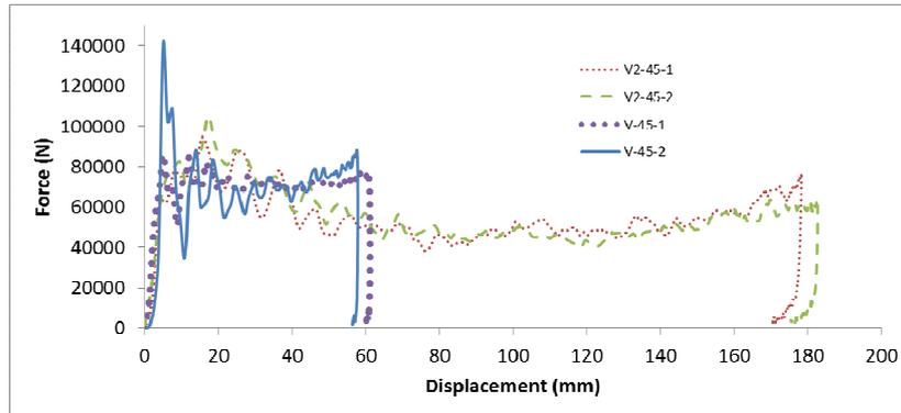
Figure 4. Force-displacement curve of the crash of composite tubes
