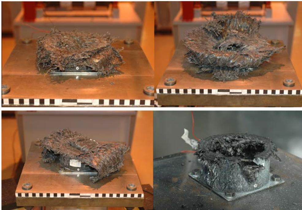
Fig. 4. Examples of crushing modes of continuous fibers composite tubes at  $0^\circ$  of impact angle: folding mode on the high left (V2-75-1), splaying on the high right (V2-20-1), splaying in 4 parts on the bottom left (V2-45-2) and fragmentation on the bottom right (C-30-1).
