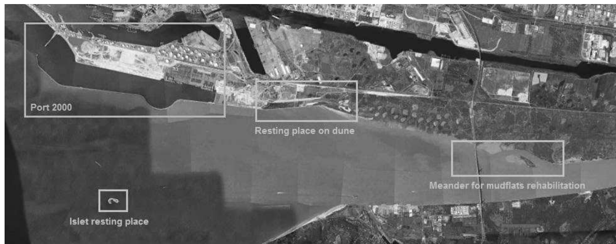
FIGURE 4 - Aerial view of Port 2000 and the environmental measures accompanying the project (Image: Google Earth - Cnes/Spot Image 2013)
