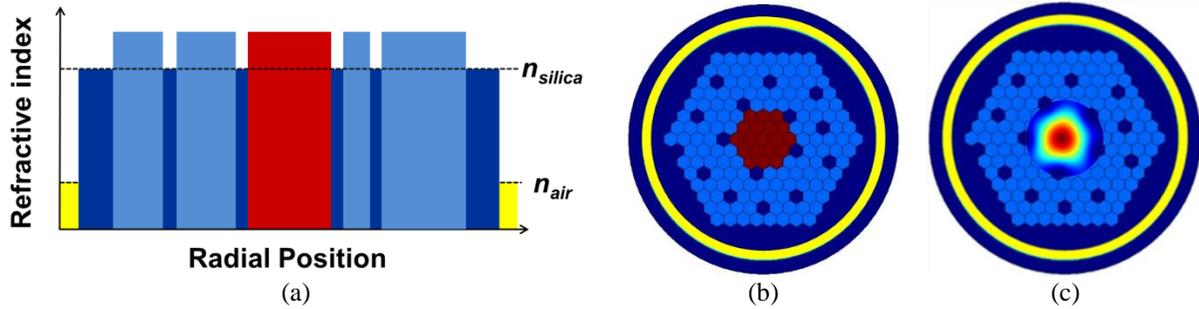
**Fig. 1:** (a) Schematic representation of the refractive index profile and (b) Cross-section of the triple-clad fully aperiodic fiber. The gain region is represented in red, the index-matched passive material in light blue, the pure silica inclusions and trench are depicted in dark blue whereas the yellow area stands for the air-clad. (c) Computed intensity distribution of the fundamental mode propagated into the FA-LPF.
