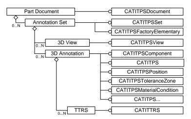
Figure 23: The object model of tolerancing components [5]
