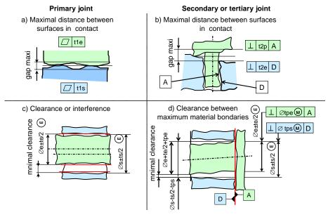
Figure 10: Positioning requirements and corresponding tolerancing
