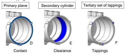
Figure 6: Selection of positioning features of the flange
