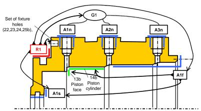
Figure 19: Links between datum reference frames
