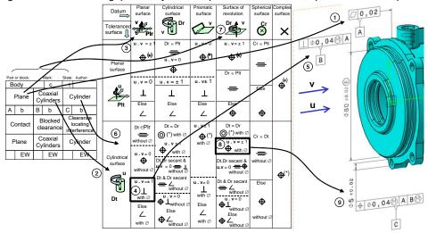
Figure 13: Specifications according to the types of toleranced surfaces and datum system
