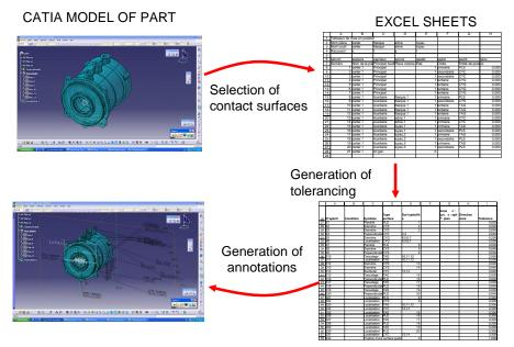
Figure 22: Interface with the CAD system
