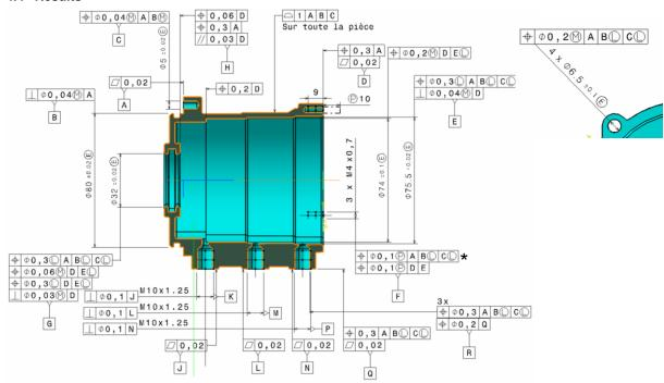
Figure 21: Complete tolerancing based on Quick GPS
