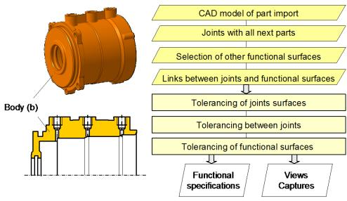
Figure 2: Tolerancing in Quick GPS
