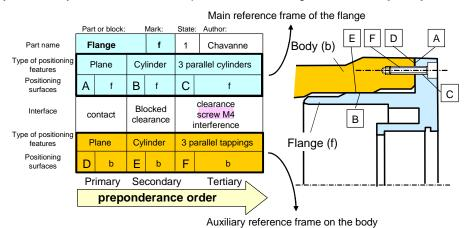
Figure 5: Positioning table of the flange
