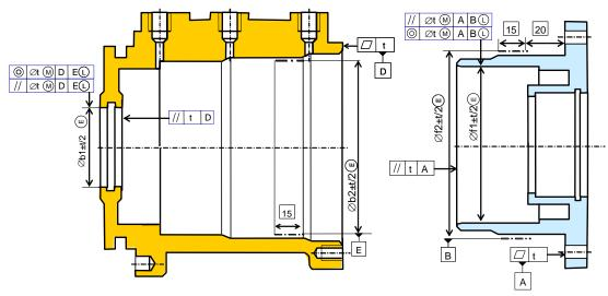
Figure 16: Breakdown of straightness into locations and orientations
