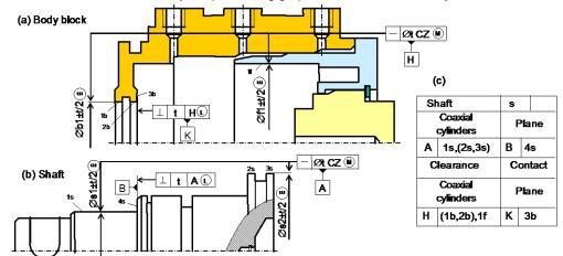
Figure 15: Straightness of both body block and shaft
