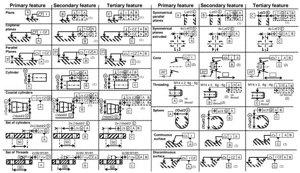
Figure 11: Patterns for positioning feature tolerancing
