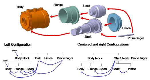
Figure 4: Two positioning graphs for the three configurations
