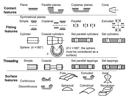
Figure 8: List of positioning features
