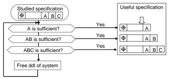
Figure 20: Test of datum frame combinations
