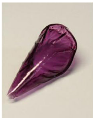
Fig. 4 PVA film containing Au NPs of 30 nm of diameter
