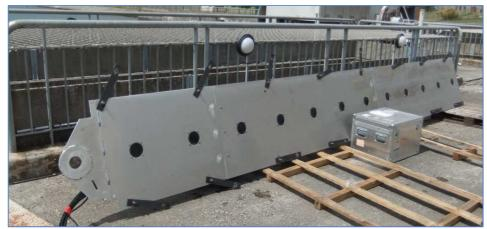
Figure 4. Steel plate carrying 12 ASFM transducers.
