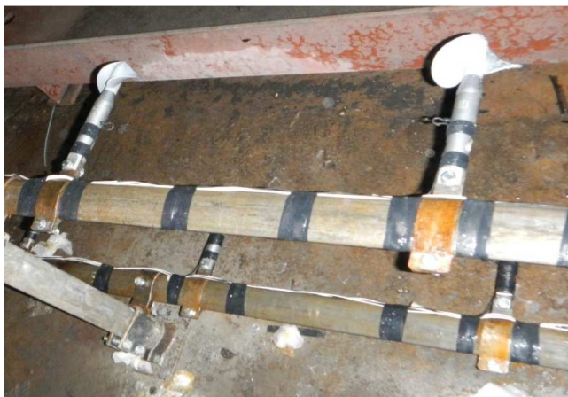
Figure 7. One of the 90 current meters used in the tests and the mounting supports on the oval section beams.
