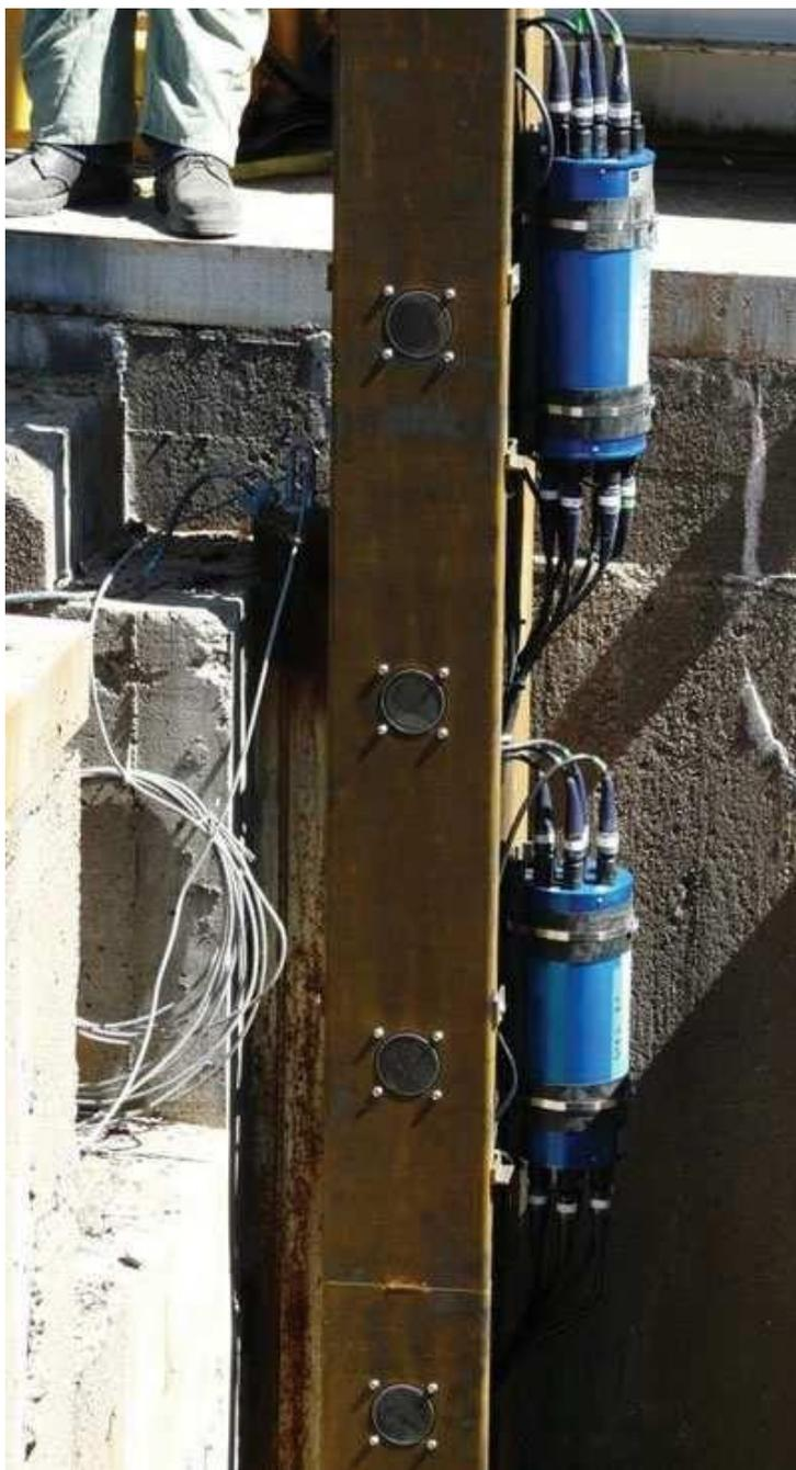
**This is a close up of horizontally installed ASFM transducers on a steel frame used for flow measurement.**
