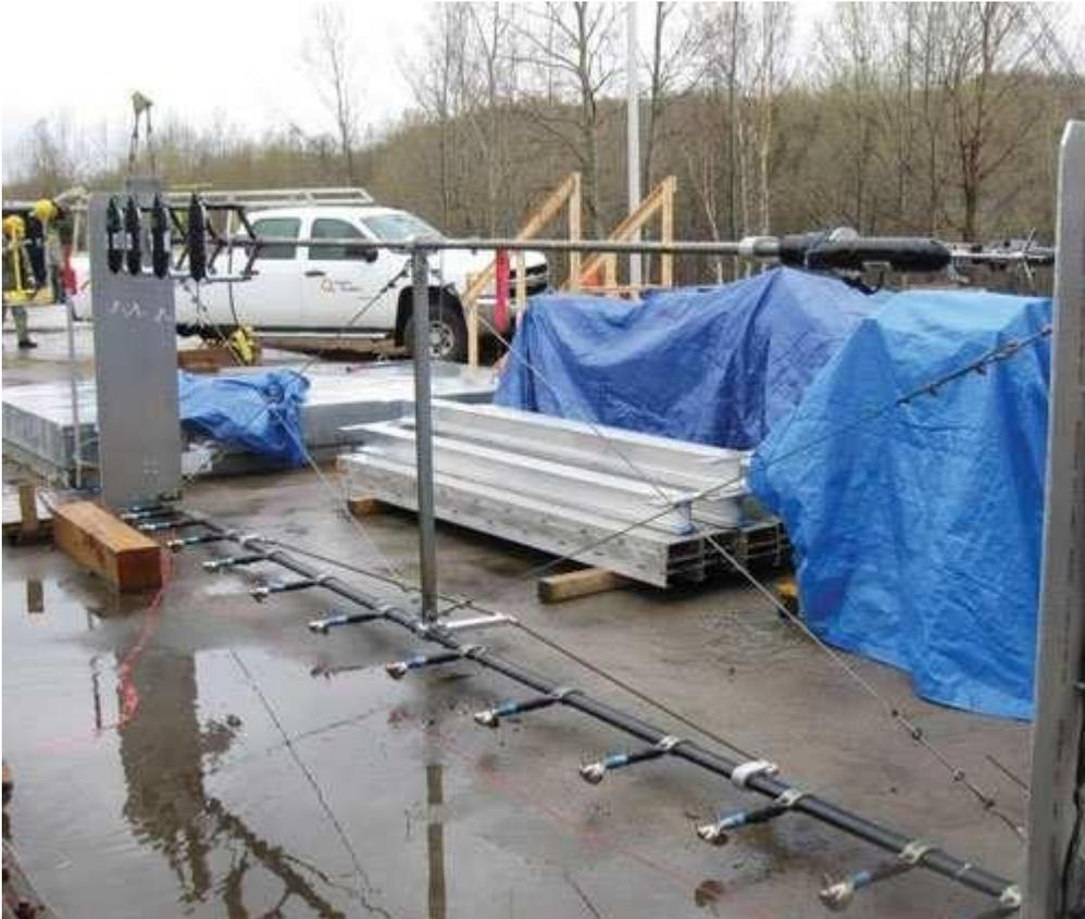
**Frame supporting the current meters. The frame had 14 current meters installed on the bottom of a simple trolley made of two end plates, profiled rods and steel cables.**
