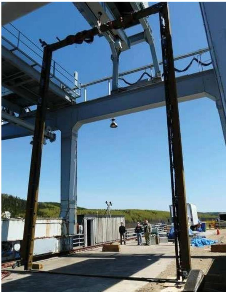
**A steel frame, which is formed by two main vertical beams, supports 21 ASFM transducers.**
