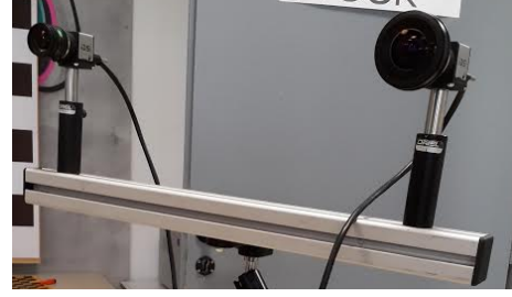
Fig. 3 Hybrid stereo-vision rig used for our evaluation
