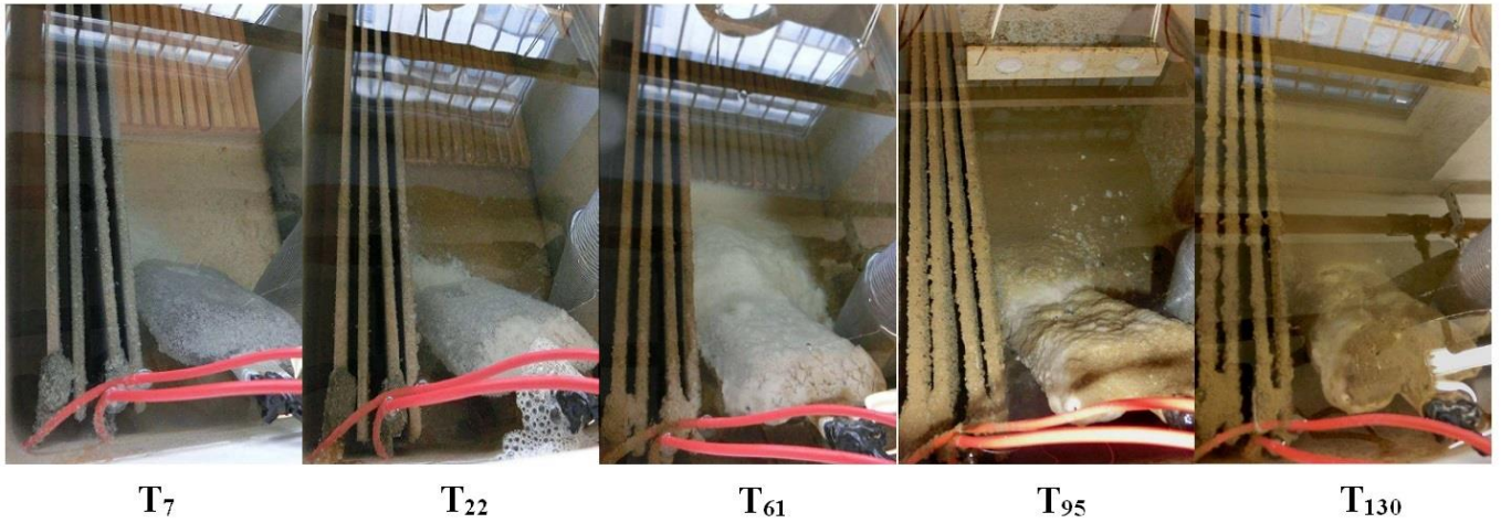
Figure 2. Dissolution of galvanic anode in the experimental tank containing steel/anode combination (S/A T) and formation of corrosion products (white layer) during the 130-day experiment.
