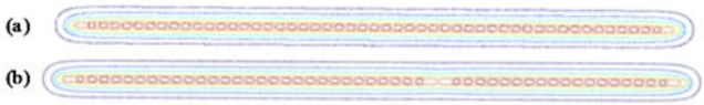
Fig. 3. Magnetic induction tangential component B x at 0.6 V-31A.: xz view of (a) a healthy cell and (b) a defective cathode channel cell
