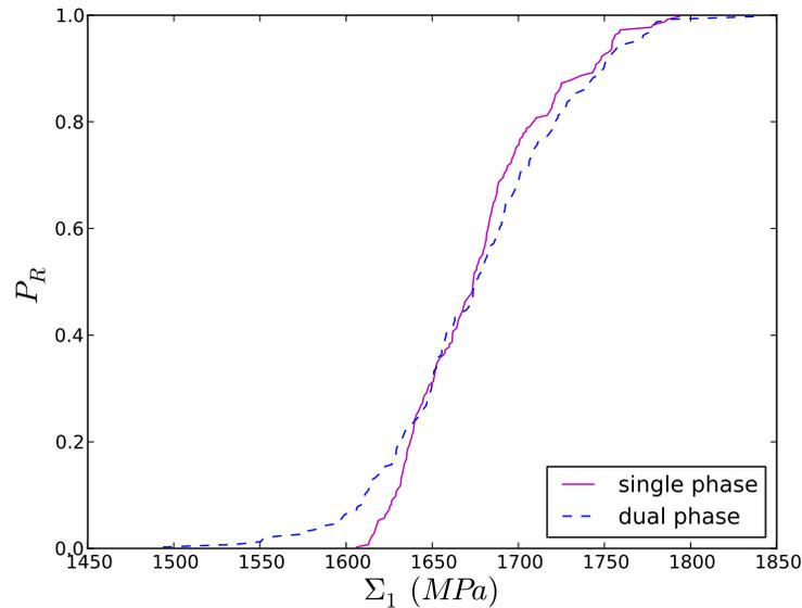
Figure 16: Failure curves of single-phase and dual-phase models at  $-150\text{ }^{\circ}\text{C}$
