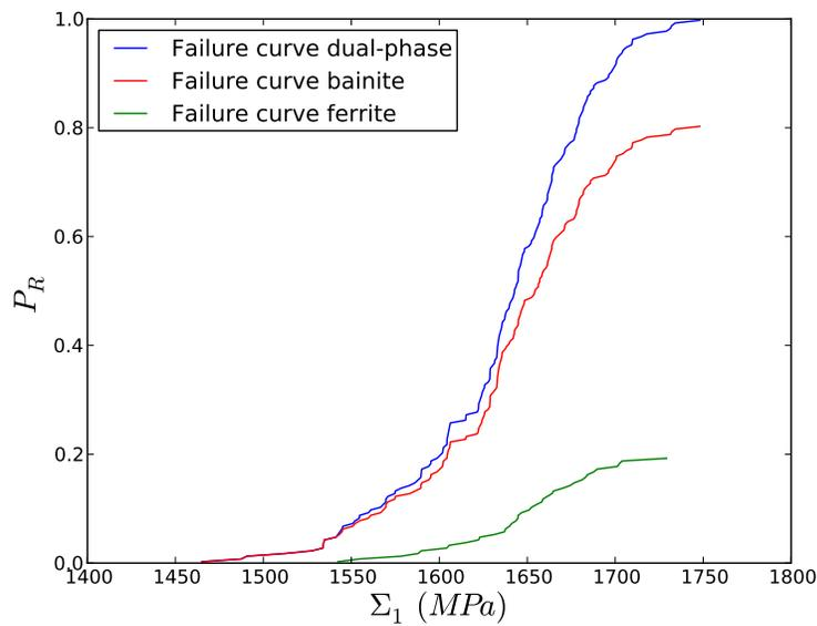
Figure 15: Failure curve calculated at  $-150\text{ }^{\circ}\text{C}$
