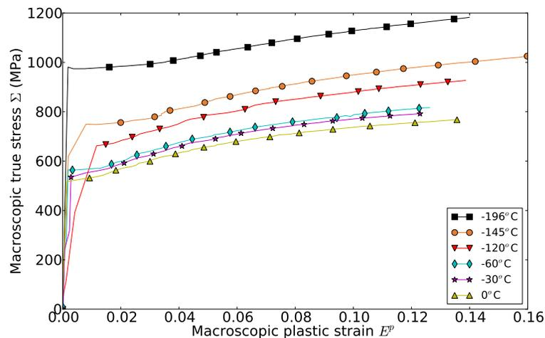
Figure 4: Stress-strain curves of 16MND5 samples of 3/4 depth, H1BQ12 material, reproduced from [25]
