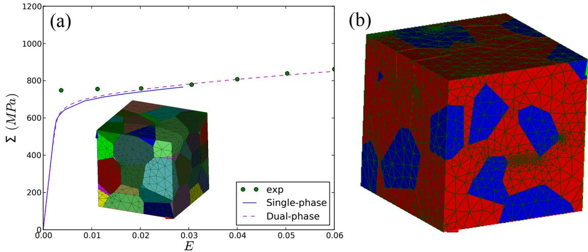
Figure 9: Macroscopic stress-strain curves at  $-150\text{ }^\circ\text{C}$  compared with experimental values (a). The meshed aggregate used to compute the tensile curves is shown with colored grains (a) and colored phases for the 75% bainite fraction case (b).
