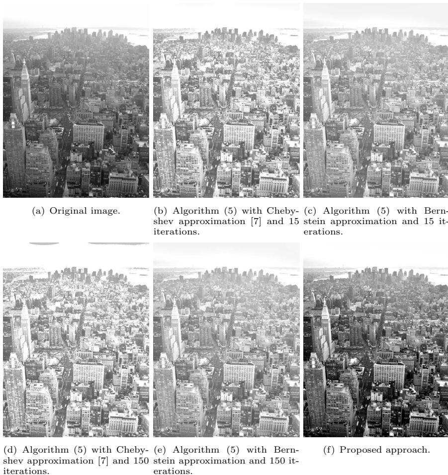
Figure 3: Comparison between the algorithm of [7] with the Chebyshev polynomial approximation and the Bernstein one after 15 and 150 iterations. Too many iterations result in over-contrasted images. The proposed approach enables to control the contrast level.
