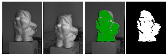
Figure 3. Creation of the mask I , determining the POI region of a scanned surface from the pair of stereoscopic images.
