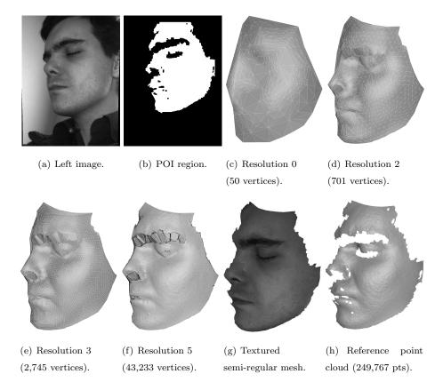
FIGURE 14: Semi-regular reconstruction of the model FACE.
