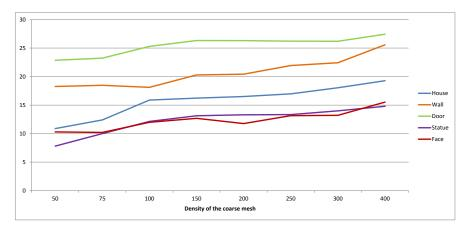
FIGURE 19: Runtimes (in sec.) of our method in function of the number of vertices of the base mesh.
