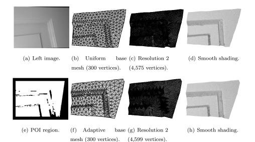
FIGURE 15: Preservation of the geometrical features of DOOR, with the uniform or the adaptive sampling.
