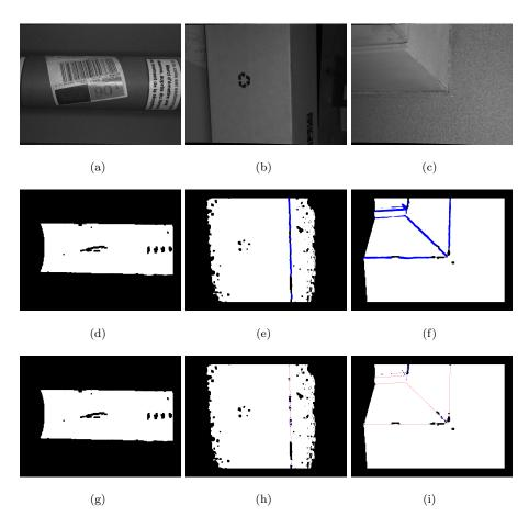
FIGURE 8: Detection of the feature lines *via* our classification technique. First row : left stereoscopic images obtained with our scanner (models PIPE, BOX and WALL). Second row : detection of high curvature areas (in blue). Third row : resulting classification after thinning : white, red and blue pixels represent respectively the *smooth regions*, the *sharp features* and the *corners*.
