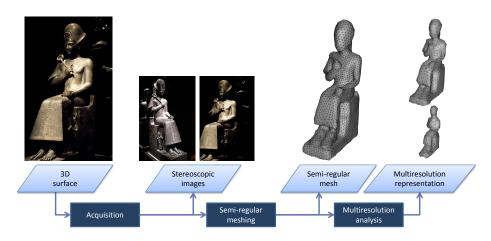
FIGURE 2: Our 3D reconstruction technique that produces a semi-regular mesh directly from stereoscopic images.
