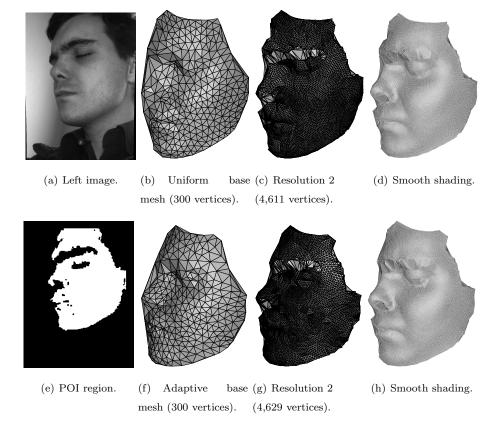
FIGURE 16: Difference of sampling quality obtained on FACE in function of uniform/adaptive sampling.
