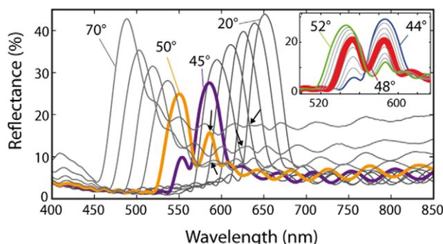
**Figure 4.** Unpolarized reflection spectra of the opal sample for incidence/reflection angles  $\theta$  ranging from  $20^\circ$  to  $70^\circ$  by steps of  $5^\circ$ . The secondary peak is indicated by arrows. (inset) Unpolarized reflection spectra for  $\theta$  from  $44^\circ$  to  $52^\circ$  by steps of  $1^\circ$ .
