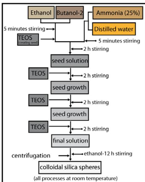
Figure 1. Process used to synthesize silica spheres.
