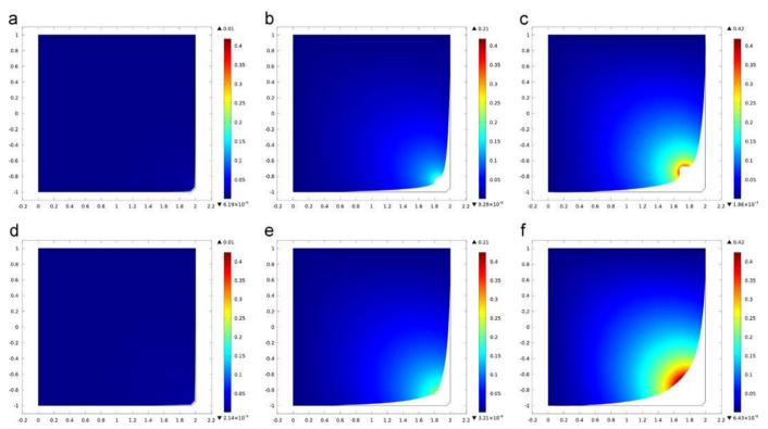
**Fig. 9.** Three snapshots of a continuum square body with an imposed motion on the right bottom vertex in direction (-1,1), in the case of a first gradient energy (a,b,c) and a second gradient energy (d,e,f). Colors represent deformations values. (For interpretation of the references to color in this figure caption, the reader is referred to the web version of this paper.)
