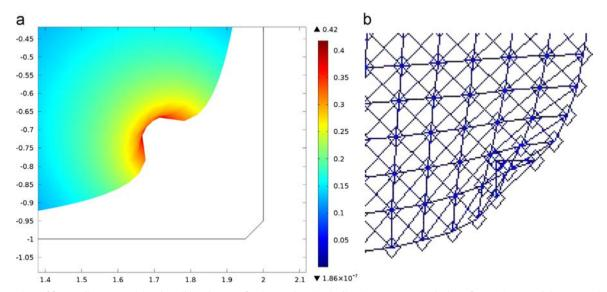
Fig. 10. Comparison of first gradient energy (a) and FNI (b) in the case of an imposed motion in direction (-1,1). Note the loss of convexity around the vertexes in both cases.
