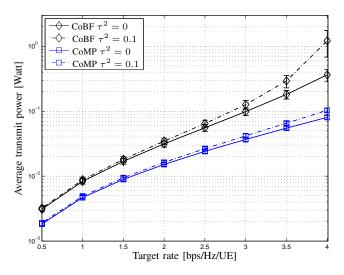
Fig. 2. Average transmit power in Watt vs. target rate when L = 16, K = 8 and N = 32.
