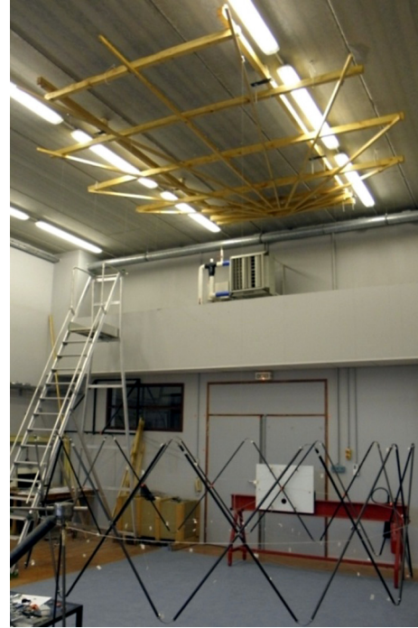
Fig. 8. The deployed prototype suspended and attached to a fixed frame.
