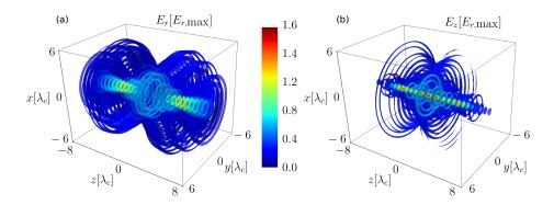
Figure 5: The absolute values of the radial and longitudinal electric fields  $E_r$  (a) and  $E_z$  (b) of a longitudinal needle beam in the focal region. The fields are normalized to the maximum  $E_{r,\text{max}}$  of the radial field  $E_r$  in the whole space.
