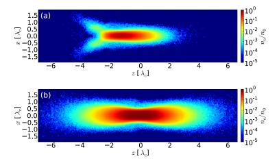
Figure 4: Electron densities  $n_e$  produced by the tightly focused Gaussian laser pulses shown in Fig. 3 (see text for details). The profile produced by paraxial LBCs (a) is even qualitatively different than the one produced by Maxwell consistent LBCs (b). Electron densities are scaled to the initial neutral density  $n_0$ . The laser propagates from left to right.
