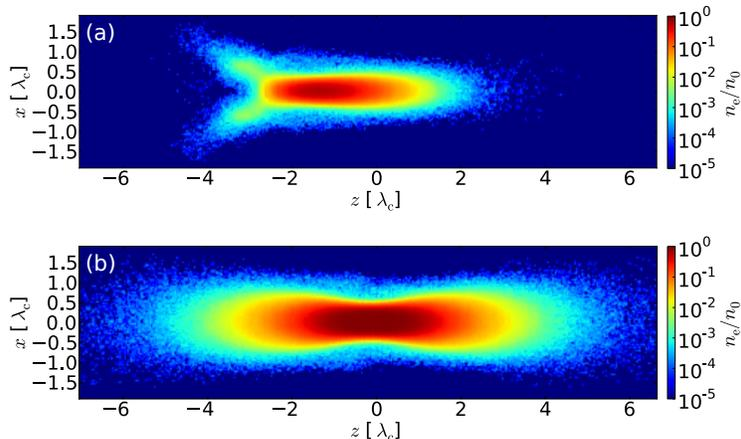
Figure 4: Electron densities  $n_e$  produced by the tightly focused Gaussian laser pulses shown in Fig. 3 (see text for details). The profile produced by paraxial LBCs (a) is even qualitatively different than the one produced by Maxwell consistent LBCs (b). Electron densities are scaled to the initial neutral density  $n_0$ . The laser propagates from left to right.
