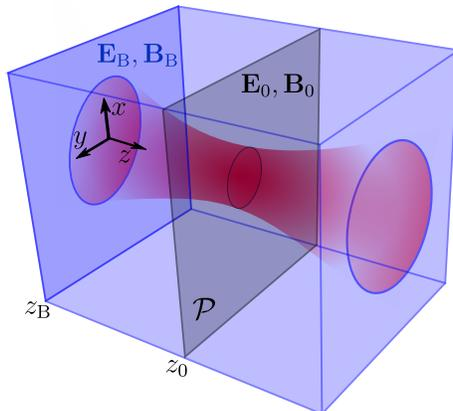
Figure 1: Schematic picture of the laser (red) injection problem into the computational domain: Electric and magnetic fields  $\mathbf{E}_0, \mathbf{B}_0$  are prescribed in the plane  $\mathcal{P}$  [here the  $(x, y)$ -plane at  $z = z_0$ ]. The fields  $\mathbf{E}_B, \mathbf{B}_B$  at the boundary (blue) are unknown and have to be calculated.
