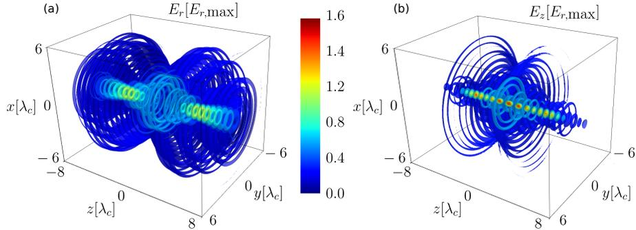
Figure 5: The absolute values of the radial and longitudinal electric fields  $E_r$  (a) and  $E_z$  (b) of a longitudinal needle beam in the focal region. The fields are normalized to the maximum  $E_{r,\max}$  of the radial field  $E_r$  in the whole space.
