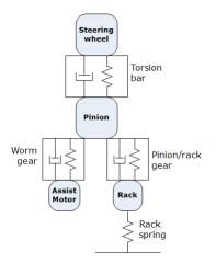
Fig. 1. P-EPS mechanical model
