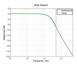
Fig. 9. Comparison between continuous PI observer and discretized PI observer at 10ms
