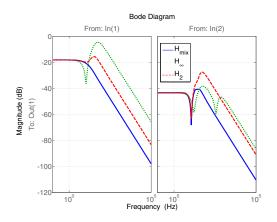
Fig. 6. Comparison between  $H_\infty,\,H_2$  and  $H_\infty/H_2$  design performance on  $T_{\bar{z}n}$
