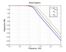
Fig. 7. Comparison between  $H_\infty,\,H_2$  and  $H_\infty/H_2$  design performance on  $T_{\hat{d}d}$
