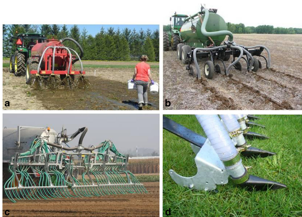
Fig. 2 Four typical methods of digestate application: splash-plate surface application (a), injection (b), trailing hose (c) and trailing shoe (d) (adapted from: Claudia Wagner-Riddle's University of Guelph team (a), extension.org (b), commons.wikimedia.org (c) and abbeymachinery.com (d))
