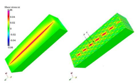
Fig. 7. Shear stress  $\tau_{xz}$  distribution (left FE result with two different homogeneous layers, right MG result with two different fiber orientation layers).
