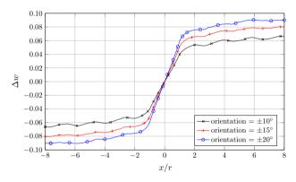
**Fig. 12.** Influence of fiber orientation on  $\Delta w$ .
