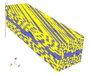
**Fig. 9.** Measured structure: yellow-fibers, light blue-matrix, dark blue-voids (top layer  $+15^{\circ}$ , bottom layer  $-15^{\circ}$ ). (For interpretation of the references to color in this figure legend, the reader is referred to the web version of this article.)
