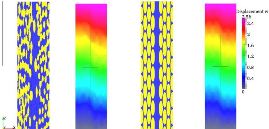
Fig. 10. Structure and displacement  $w$  distribution at the boundary surface:  $y = -32r$  for the real case and the ideal case (interface layer thickness =  $2r$ ) respectively (from left to right: real structure, displacement  $w$  distribution for the real case, ideal structure, displacement  $w$  distribution for the ideal case).
