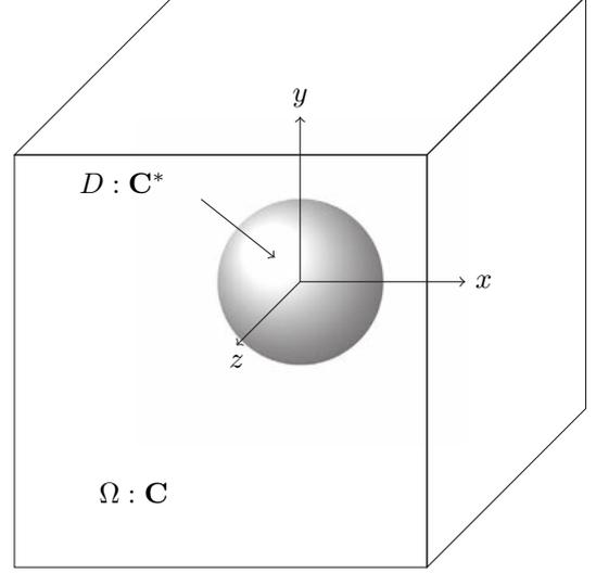
Fig. 2. Cubic matrix containing a spherical inhomogeneity.
