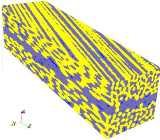
Fig. 9. Measured structure: yellow-fibers, light blue-matrix, dark blue-voids (top layer  $+15^\circ$ , bottom layer  $-15^\circ$ ). (For interpretation of the references to color in this figure legend, the reader is referred to the web version of this article.)
