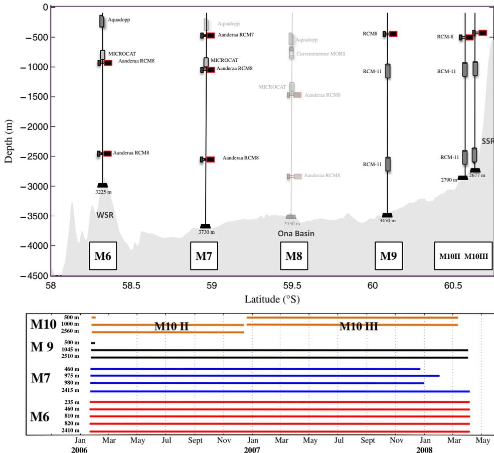
**Figure 3.** (top) Distribution of the mooring lines and instruments. Mooring M8 (half-toned) was lost. The South Scotia Ridge (SSR) and West Scotia Ridge (WSR) are labeled. (bottom) measurement calendar.
