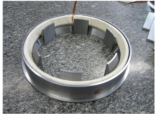
Fig. 5. Prototype: One half of claw pole stator yoke
