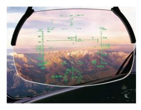
Fig. 3. Close-up view of the Boeing 787 head up display
