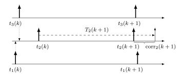
Fig. 1. Round k and k+1 pulses of a three node system. Node 2 adapts the time of occurence of its round k+1 pulse by a negative offset  $corr_2(k+1)$ due to the early pulses received from nodes 1 and 3.
