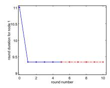
Fig. 4. Prefix of an execution of a diffusive algorithm with fixed weights run in the example dynamic network of Fig. 3. Solid lines represent rounds k at which  $G(k) = G_1$ , and dotted lines those where  $G(k) = G_2$ .
