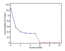
Fig. 3. Prefix of an execution of the example dynamic network for rounds  $0 \le k \le 10$ . The communication graph changes from  $G_1$  (solid lines) to  $G_2$  (dotted lines) at round 5. The figure shows (i) pulse generation times  $t_i(k)$ , (ii) maximum phase differences  $\max_{i,j} |t_i(k) - t_j(k)|$ , and (iii) round durations  $t_1(k+1) - t_1(k)$ .
