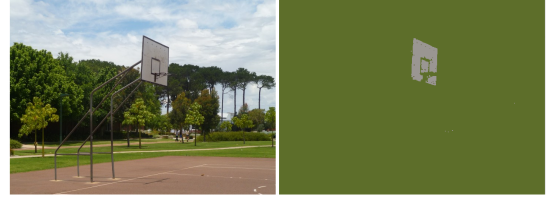
Figure 7: Segmentation of a natural scene. On the left, the original image where a color sample was taken from the white backboard. On the right, the segmentation achieved.
