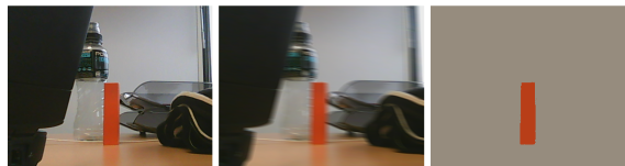
Figure 8: Segmentation under camera motions. On the left, the still image of the scene. In the center, a random motion was applied to the camera. On the right, the segmentation obtained.
