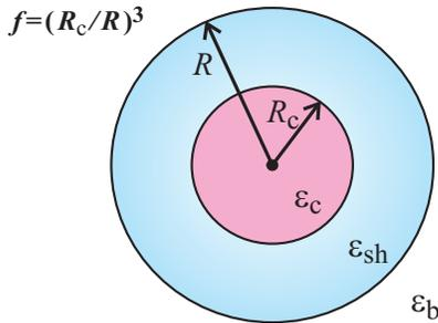
FIG. 6. Schematic of a concentric coated sphere where the core, shell, and background permittivities are denoted respectively  $\epsilon_c$ ,  $\epsilon_{sh}$ , and  $\epsilon_b$ . The filling fraction of the core material is defined as  $f \equiv (R_c/R)^3$ .
