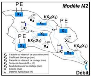
Figure 1: Spatial discretization and functioning of the GRSD model. From Lobligeois [2014].
