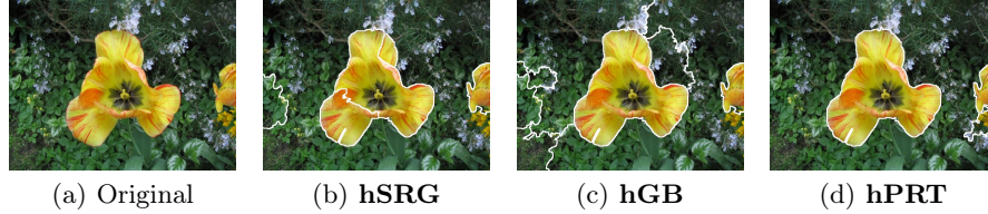
Fig. 4. Some results by using the hierarchical compared segmentation methods ( hGB , hSRG and hPRT ). In order to compute these results, we consider the parameters that makes possible to obtain the yellow flowers (center and right of the original image).
