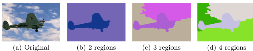
Fig. 2. A real example illustrating the hierarchical segmentation obtained by our proposed method inspired by similarity measure proposed in [17] showing the number of regions. Moreover, the location of the contours are stable in different segmentations.
