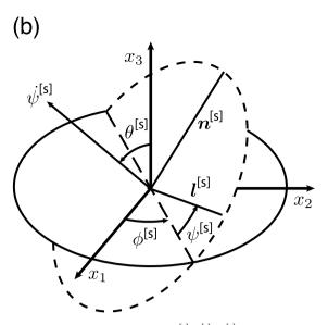
**Figure 2.** (a) General definition of the Eulerian angles  $(\phi, \theta, \psi)$ . (b) Definition of slip-system specific Eulerian angles  $(\phi^{[s]}, \theta^{[s]}, \psi^{[s]})$  such that both the slip direction  $I^{[s]}$  and the normal  $n^{[s]}$  to the slip plane are in the plane perpendicular to the  $\dot{\psi}^{[s]}$ -axis.
