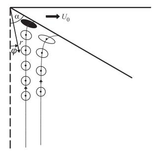
**Figure 9.** Geometry and boundary conditions for the corner flow model of a ridge crest (right half only). The half spreading rate is  $U_0$  and the asthenospheric wedge has angular dimension  $\alpha = 60^{\circ}$ . Solid lines with arrows show typical streamlines for a power-law rheology with index n = 3. The FSEs are plotted at different points along the two streamlines. The black ellipse relates to the point in the flow at which the texture is approximated (see Fig. 10).
