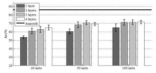
Figure 1: Phone recognition accuracy according to the number of layers and the number of units per layer using DNN-based mapping (mean±SD). The thick line represents the recognition accuracy on original audio.
