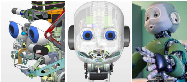
Figure 3. Details of the iCub talking head. Removable eye caps are highlighted in blue. Left: four motors are shaping the lips. The lower lip is carried by the jaw. Center: the skull and jaw consist of two rigid covers. Right: Nina’s final appearance.
