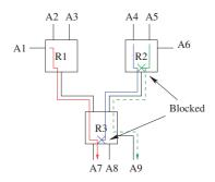
Fig. 1. Wormhole routing
