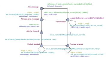
Fig. 2. Timed automaton of an outport of a router
