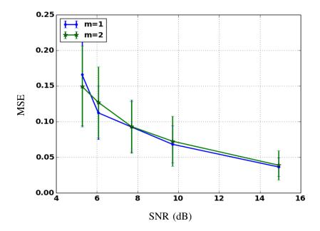
Fig. 6. Evolution of the mean MSE and standard deviation on estimated NRLs with JPDE, for 5 different input SNR values and for the two experimental conditions.
