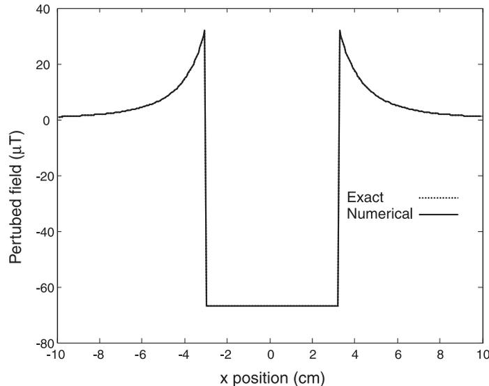
Figure 4. Magnetic field perturbation along a scan line oriented in a direction orthogonal to the magnetic field  $\mathbf{B}_0$  (1 T.) and passing through the center of a paramagnetic ball ( $\chi_m = 4 \cdot 10^{-3}$ ) of radius 3 cm. The numerical computation is done using 10080 triangles for the mesh of the ball surface.
