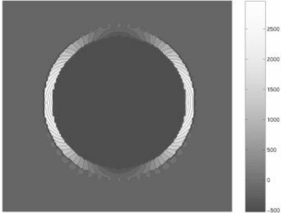
Figure 9. Induced magnetic field (in  $\mu T$ ) on a central slice parallel to  $\mathbf{B}_0$  for a hollow ball associating titanium ( $\chi_m = 23 \cdot 10^{-4}$ ) and bismuth ( $\chi_m = -11.9 \cdot 10^{-4}$ .)
