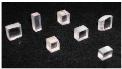
Figure 1: Czochralski □-BBO grown in super cooled melt (left). Samples are sawn from clear and less stress part of the bowl. Oriented and polished sample (right).
