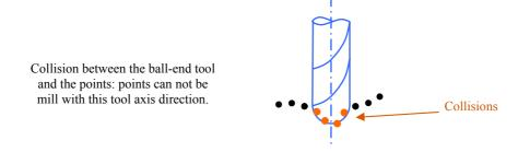
Figure 6. Collisions between the ball-end tool and the point cloud.
