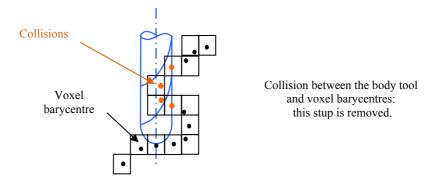
*Figure 8. Collisions between the tool and the barycentres.*
