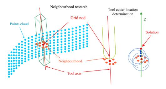
Figure 3. Tool cutter location on discrete data
