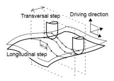
Figure 2. Tool path generation
