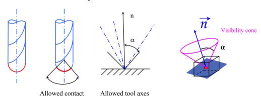
Figure 7. Determination of the visibility cone
