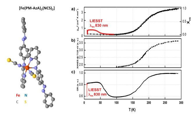
**FIG. 1.** Thermal spin crossover of the [Fe(PM-AzA)<sub>2</sub>(NCS)<sub>2</sub>] compound (top) monitored with the evolution of **a**)  $\chi_M$ .T product, **b**) X-ray absorption at 7125 eV, **c**) total optical reflectivity. The increase of  $\chi_m$ .T and OR under cw light excitation at 830 nm in a) and c) is related to the long-lived LIESST phenomenon at low temperature.
