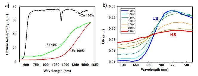
**FIG. 2. a)** diffuse reflectivity spectra collected on powders of  $[Fe(PM-AzA)_2(NCS)_2]$  (—),  $[Zn_{0.9}Fe_{0.1}(PM-AzA)_2(NCS)_2]$  (—) and  $[Zn(PM-AzA)_2(NCS)_2]$  (—) crystals. **b)** optical reflectivity spectra of a  $[Fe(PM-AzA)_2(NCS)_2]$  single crystal acquired at different temperatures during the SCO from pure LS (100 K) and HS (270 K) states.
