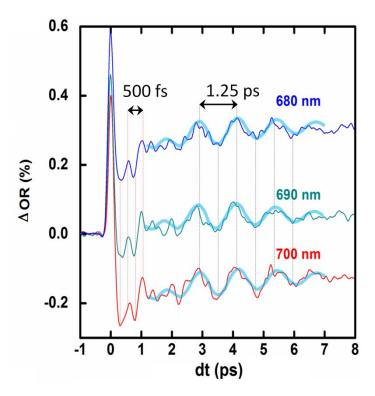
**FIG. 6.** Dynamical OR time traces recorded at 680 nm 690nm and 700 nm after photoexcitation at 800 nm (0.4 mJ/mm<sup>2</sup>) and showing in phase oscillations of the reflectivity signal Thick cyan curves represents the fit to the data with a sine function multiplied with an increasing and decreasing exponential terms
