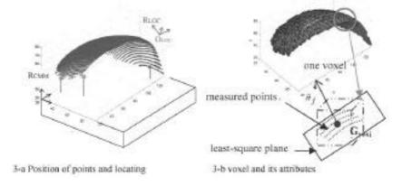
Figure 3: Measured points and voxel representation
