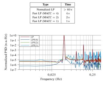
Fig. 4. Comparison of raw implementation of Lomb-Scargle (LP) and its fast implementation LPF(1), LPF(2) and LPF(4), for a 0.05 Hz triangular modulation of HR.
