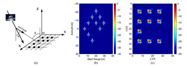
Fig. 4. Refocusing Algorithm Simulation. (a) Simulation scenario. (b) Focused SAR image with the Frequency Scaling Algorithm in slant range-azimuth geometry. (c) Refocused image on a grid placed in the horizontal plane containing the scatterers.
