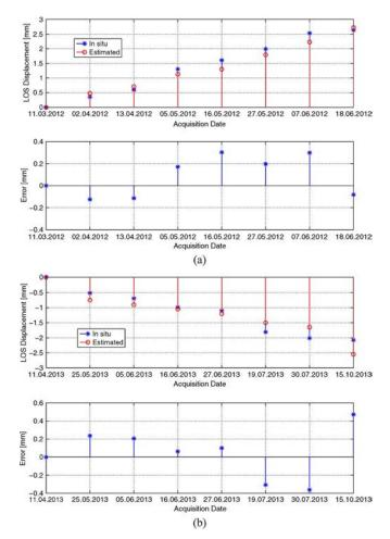
Fig. 18. Estimated versus *in situ* LOS displacements between two regions of the Puylaurent dam for the two data sets: (a) May–June 2012, (b) April–October 2013.
