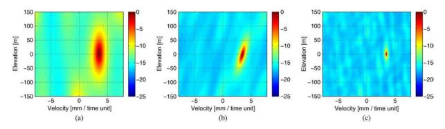
Fig. 10. Estimated EV PSD planes for a SNR of 10 dB and different number of satellite passes (a) 5 tracks, (b) 8 tracks, and (c) 15 tracks.
