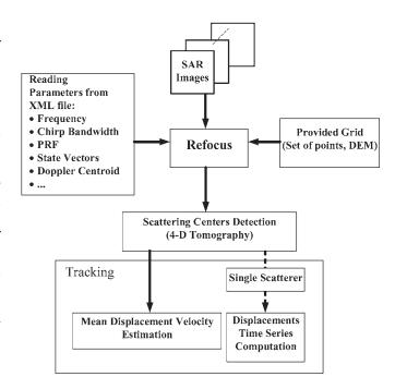
Fig. 1. Scattering centers detection and tracking based on SAR images refocusing.
