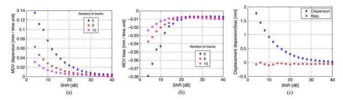
Fig. 8. (a) Dispersion of estimated MDV, (b) bias of estimated MDV, and (c) displacement dispersion/bias versus SNR for one scatterer with linear motion in LOS.
