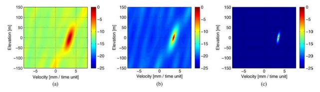
Fig. 9. Estimated EV PSD planes for eight tracks and different SNRs (a) 5 dB, (b) 15 dB, and (c) 25 dB.
