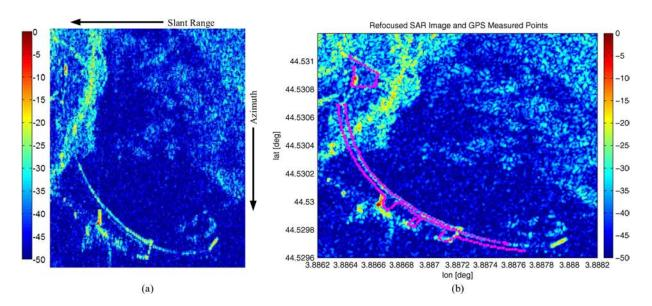
Fig. 14. Two-Dimensional Grid Refocusing. (a) High-Resolution Spotlight TerraSAR-X SAR image of the Puylaurent dam acquired on March 11, 2012. (b) Refocused TerraSAR-X image on the rectangular grid overlaid by the set of GPS measured points on the ridge of the dam.
