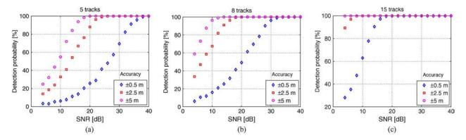
Fig. 7. Detection probability versus SNR for one scatterer having a linear motion in LOS. The considered accuracies are 0.5 m, 2.5 m, and 5 m and the number of simulated satellite passes are (a) 5 tracks, (b) 8 tracks, and (c) 15 tracks.
