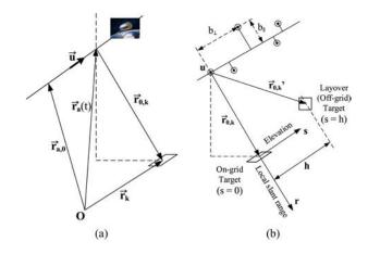
Fig. 3. (a) Refocusing geometry for a target with a known on-grid position  $\vec{r}_k$ . (b) Layover detection geometry based on zero elevation for on-grid targets.
